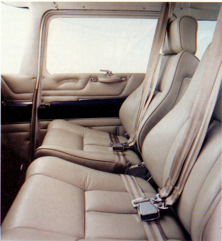
Shoulder harnesses, such as these B.A.S. Inc. harnesses with inertia reels (above) installed in a Cessna 172, are an excellent starting point for modifying a Cessna 182. Also popular are engine upgrades; Air Plains Services, of Wellington, Kansas, offers 300-horsepower conversions for 182s that utilize one of two Continental powerplants (top and preceding pages).
