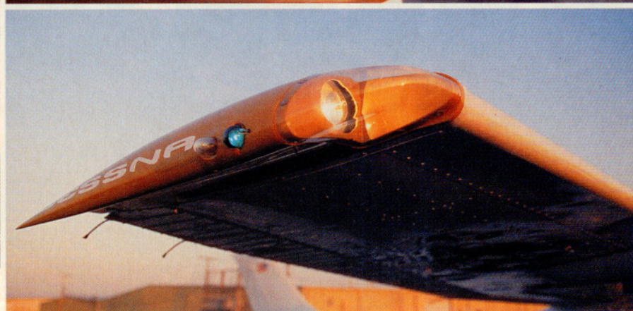
All of Air Plains Services' Cessna Skylane engine upgrades include three-blade Hartzell propellers (above left). Exhaust stack extensions (top) from Texas Skyways and wingtip recognition lights (above) from RMD Aircraft Lighting are among many other available mods. A Horton STOL kit, shown for a Cessna 172 (bottom, facing page), includes distinctive drooped wing tips.
